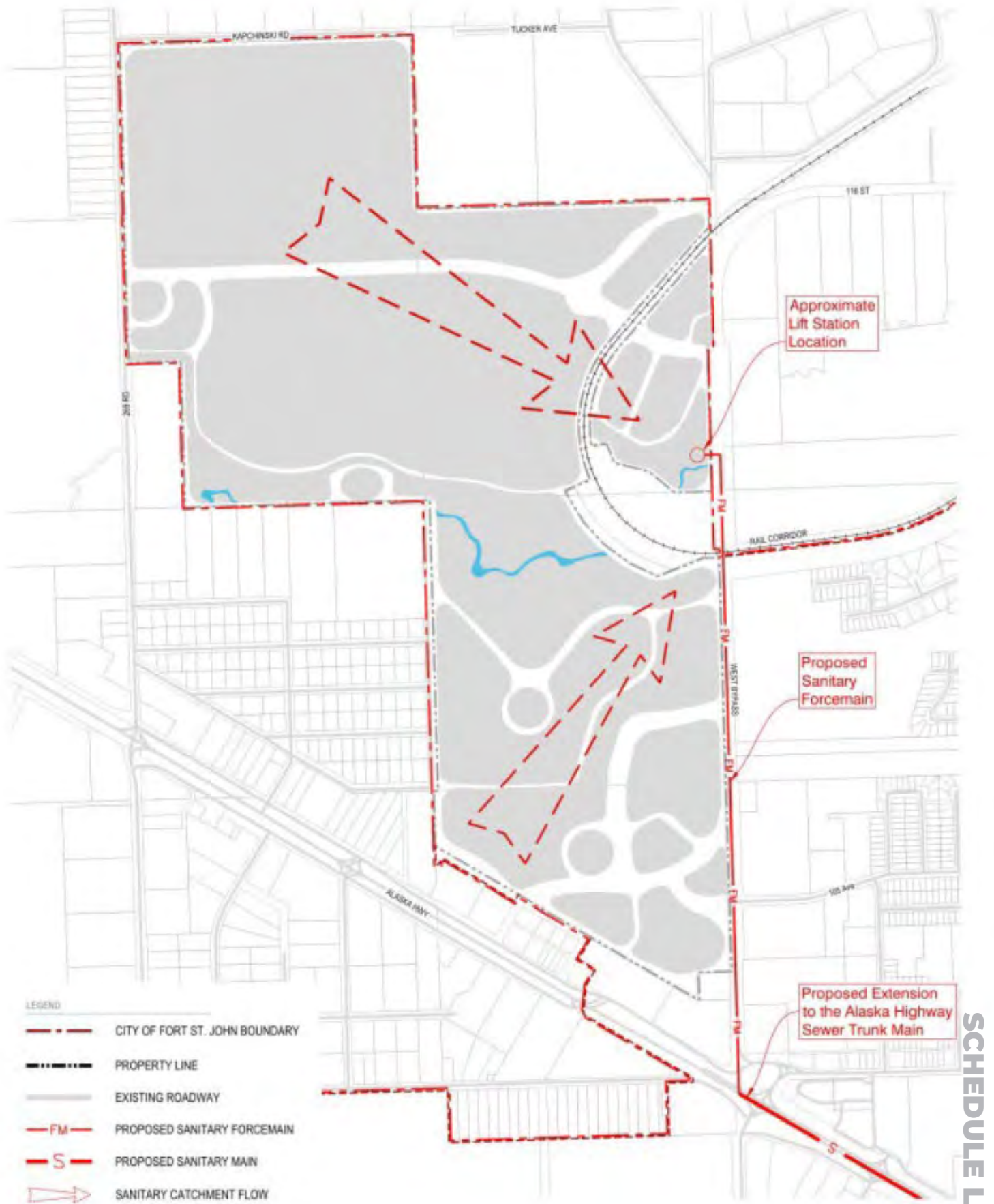
Figure 3: Sanitary Sewer System
